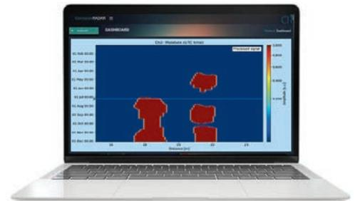
**CorrosionRADAR** moisture sensor data analysis and correlation with historical weather data.
